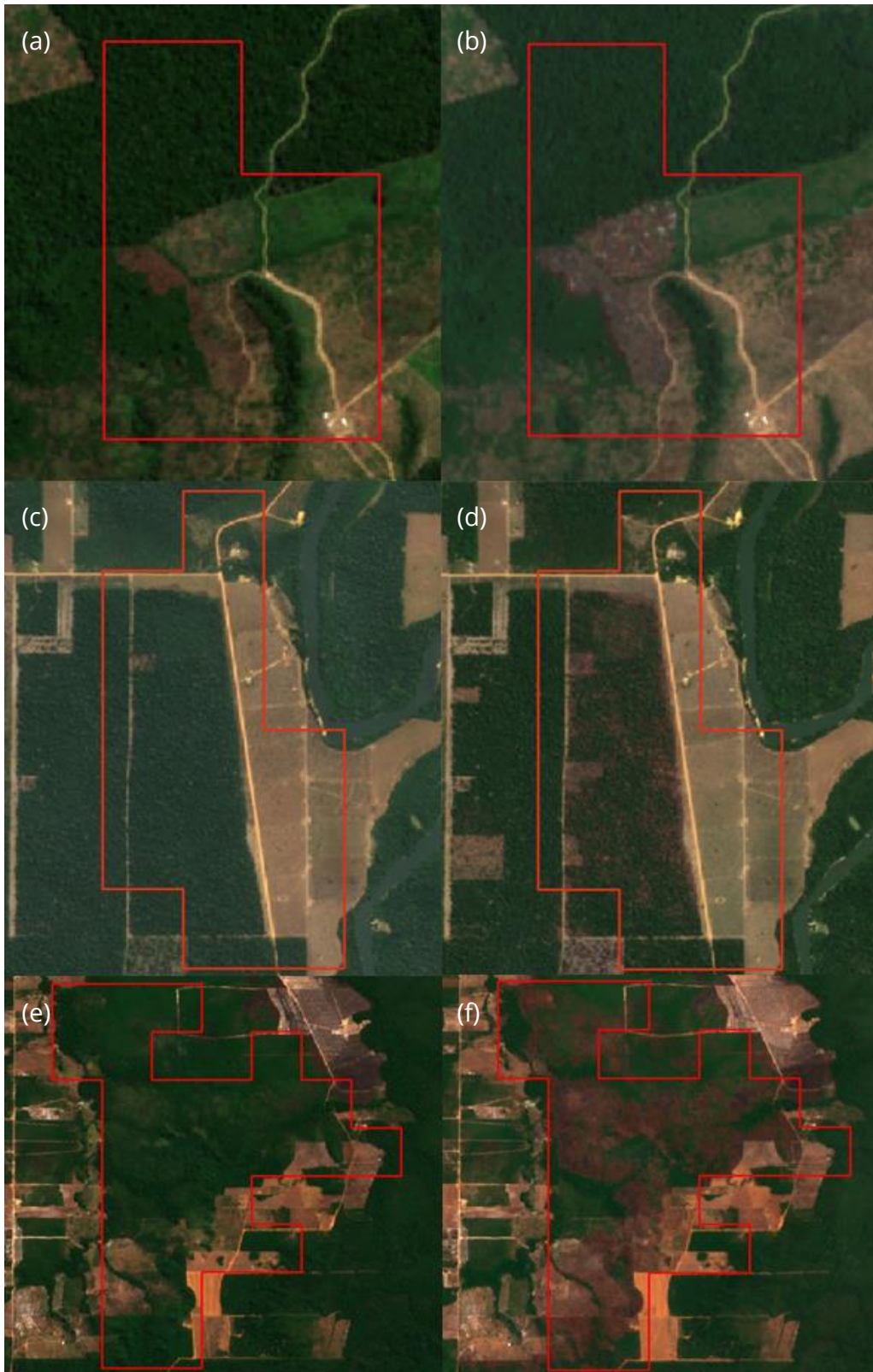
Figure 1: Example highlighting how fire type can be interpreted from 10-m resolution pre- and post-fire Sentinel-2 image pairs.
